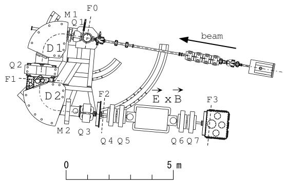
Fig. 1. Plane view of CRIB. Primary low-energy heavy-ion beams are provided from the AVF cyclotron of RIKEN.
